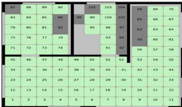
**Figure 2.** A cartography of the tiles composing the sensing floor, with their identifiers.
